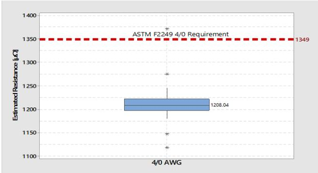
Figure 1: 4/0 TPG Measured Resistances
