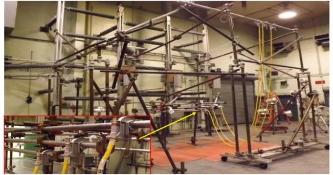
Figure 2: Test setup for three TPGs in parallel with return bus configuration to measure split currents
