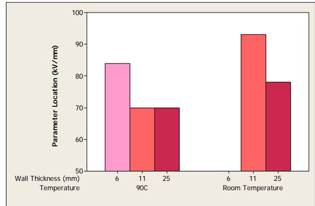
Figure 3 Effect of cable size (wall thickness) and temperature on the impulse breakdown strength of XLPE cables
