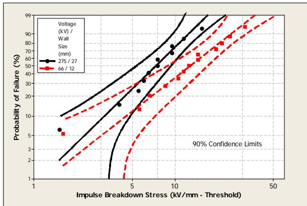
Figure 2 Effect of cable voltage and insulation thickness on the impulse breakdown strength of XLPE cables at 90°C
