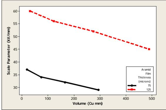
Figure 4 Effect of volume (mm<sup>3</sup>) on the breakdown stress of Aramid films.
