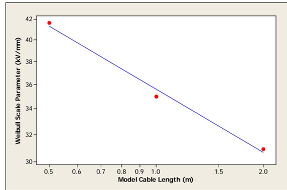
Figure 7 Reduction of breakdown strength (Figure 5) with increasing cable length
