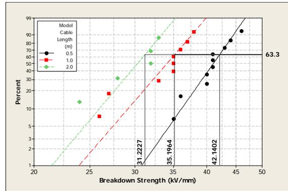
Figure 6 Breakdown strength of model cables (1.5mm wall) of different lengths after wet ageing for 1000hours
