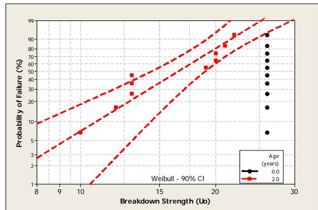
Figure 8 Breakdown strength of MV cables (20kV) after 2 years ageing
