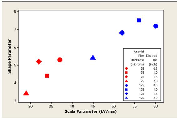
Figure 5 Full Weibull Parameter for selected thickness and electrode size
