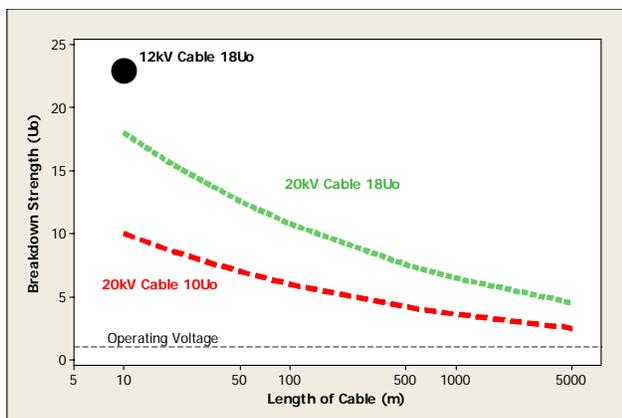
Figure 9 Effect of cable length (between joints) on the breakdown strength
