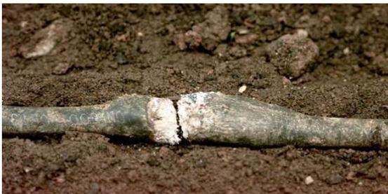
**Figure 1: Corrosion Failure**
