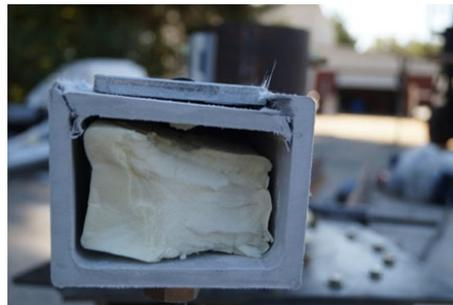
Fig. 4. Crush failure of a beam
