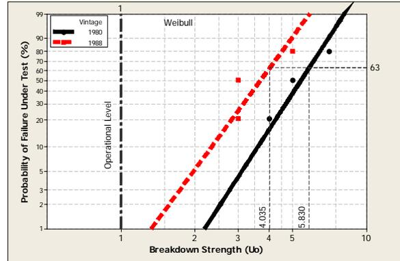
**Figure 5** AC Step ( $U_0/5\text{min}$ ) Breakdown Tests On XLPE Unjacketed Cables Identified As Poor Performers. Vertical Dashed Lines Show The Weibull Scale Parameter.
