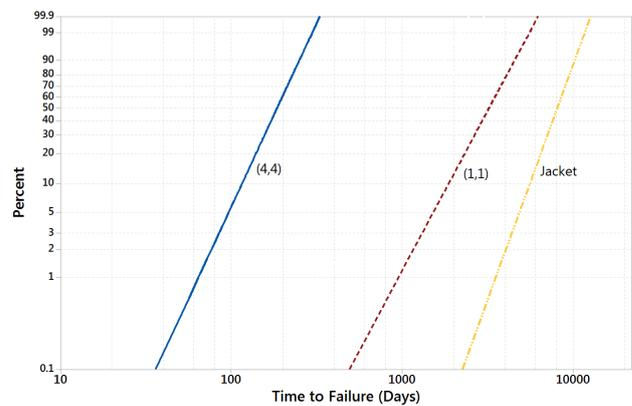
**Figure 8. Case 1 Weibull curves (adjusted scale and shape parameter) for life expansion factors. Curves move right (longer life) as expansion factors applied.**
