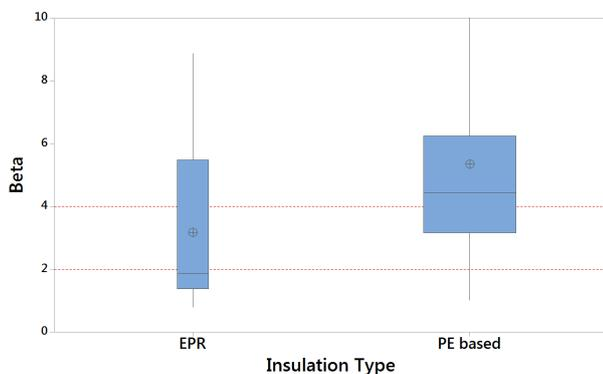
Figure 3. Boxplot of the shape parameters by insulation type – median given by central line within box.
