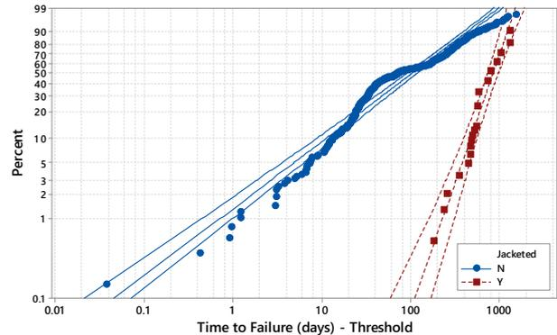
Figure 7. Weibull analysis of un-jacketed and jacketed ACLT data.
