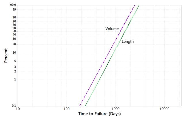
**Figure 9. Case 1 Weibull curves (adjusted scale and shape parameter) for life reduction factors. Curves move left (shorter life) as reduction factors applied.**
