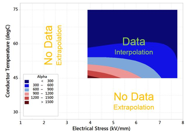
Figure 4. Illustration of using contour plot for data interpolation / extrapolation for XLPE data as.
