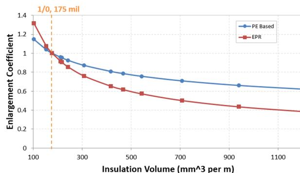
Figure 6. Enlargement coefficient for insulation volume adjustment.
